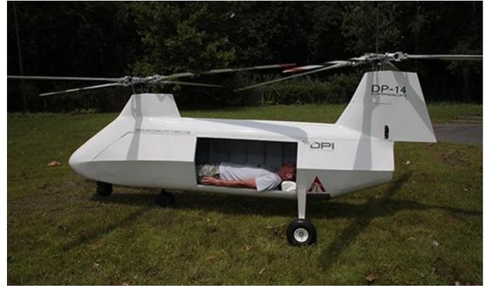
Figure 4-6. The DP-14 Designed to Carry 430-lb Useful Payload With a Large 23-ft<sup>3</sup> (Over 6 ft Long and 10 in Wide) Internal Cargo Area (Source: Dragonfly Pictures Inc. [78]).
