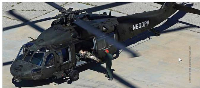
Figure 1-5. Autonomous Black Hawk With Medical Resupply and Simulated Casualty With Remote Monitoring During PC22 (Source: Fricks [15]).
