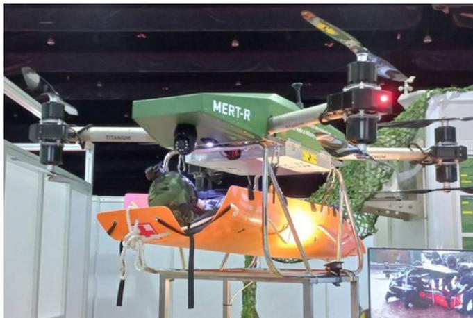
Figure 4-8. MERT-R MEDEVAC UAV Designed to Carry a Patient to a Medical Facility (Source: Nonthasa [86]).
