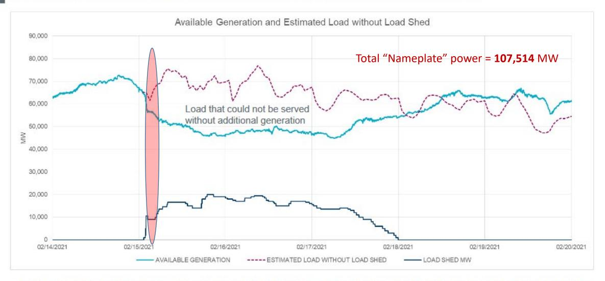
Available Generation shown is the total HSL of Online Resources, including Quick Starts in OFFQS. The total uses the current MW for Resources in Start-up, Shut-Down, and ONTEST.
