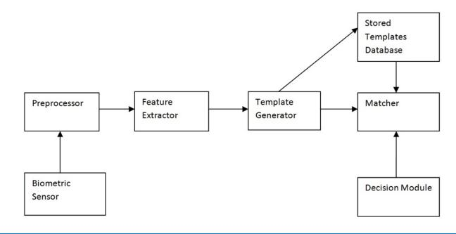
Figure 2-2. Simple Diagram of a Biometric Recognition System, Including Matching to Database of Template References [10].
