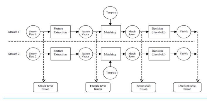
Figure 3-3. Sensor, Feature, Score, and Decision Level Biometric Data Fusion Levels [32].
