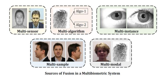
Figure 3-2. Five Sources of Information Fusion in a Multibiometric System [25].
