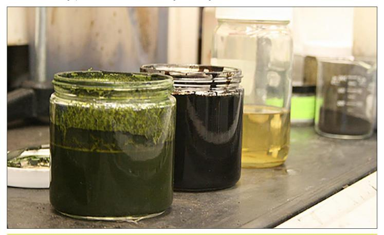
Figure 3: (L-R): Algae slurry; biocrude oil; and, with further processing, refined biocrude which contains mostly the makings of gasoline and diesel fuel. (Source: Pacific Northwest National Laboratory)
