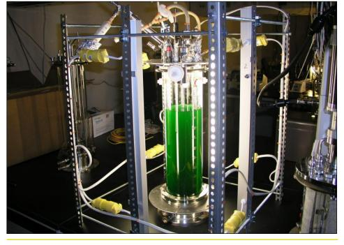
Figure 6: Synechococcus sp. PCC 7002 in a bioreactor [5].
