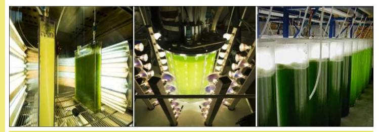
Figure 4: Closed systems. Pictures showing different types of commercially available photobioreactor systems: bags, tubular, vessels etc. (Image courtesey of Robert Henrikson)
