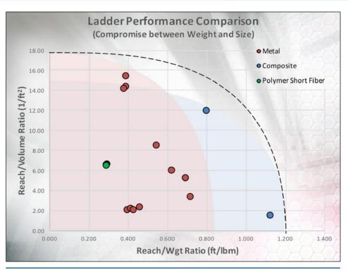
Figure 1: State-of-the-art ladders present a compromise between low weight and small collapsed size. Carbon composites push the frontier toward lower weight but are not as compact when stowed as the best metal designs.
