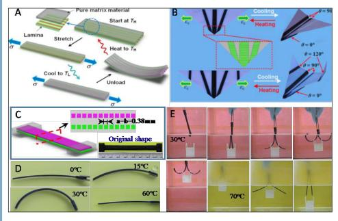
Figure 2: 4-D printing of SMP composites. (A) Schematic of the design, programming step, and shape memory cycle of a single-layer fiber-matrix composite [2]. (B) Active origami airplane utilizing the active hinges [33]. (Released) (C) The design of the composite structure with two layers of different SMP fibers embedded inside the rubbery matrix. (D) The shape changing behavior of the printed and programmed composite at different temperatures. (E) A smart hook application of the SMP composite.
