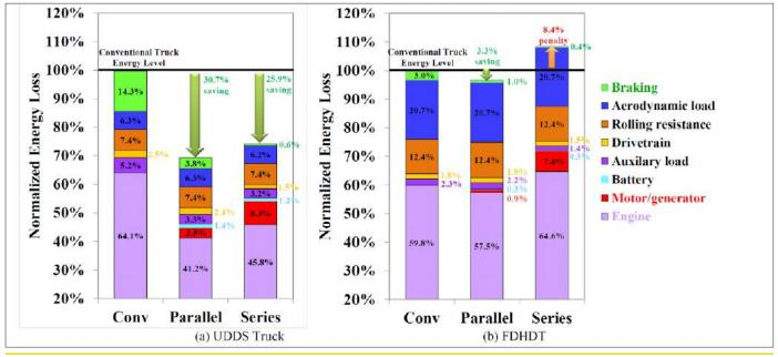
Figure 3: Normalized energy loss comparing conventional, parallel hybrid and series hybrid vehicles over urban dynanometer driving schedule and freeway-domanant heavy duty truck test cycles. [8] (Released)
