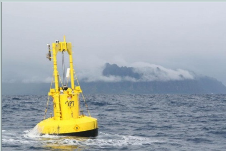
The Powerbuoy. The next generation of renewable energy technologies floats three-fourths of a mile off the north east coast of Oahu, Hawaii. Ocean Power Technologies Inc., in conjunction with Marine Corps Base Hawaii, is testing renewable energy sources for the Marine base. (U.S. Marine Corps photo by Cpl. Jody Lee Smith/Released)
