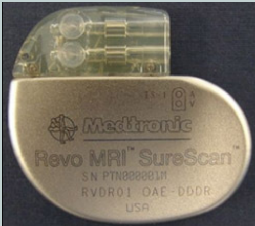
The Revo MRI SureScan Pacing System delivers standard pacing therapy to patients with slow heart rates. This particular pacemaker permits patients meeting certain criteria to receive MRI scan. (Courtesy of the U.S. FDA / Released)
