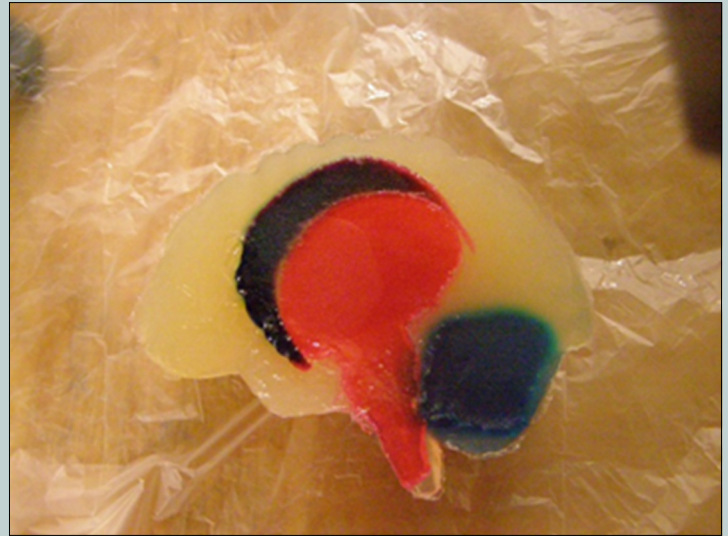
Figure 6. Photograph of the gelatin-agar brain phantom. (Released)
