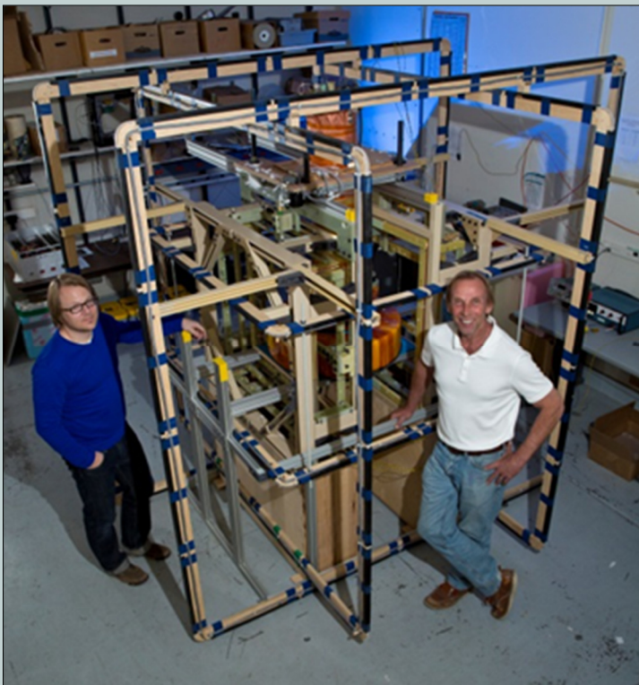
Figure 5. The Los Alamos Battlefield MRI prototype. (Courtesy of LANL/Released)
