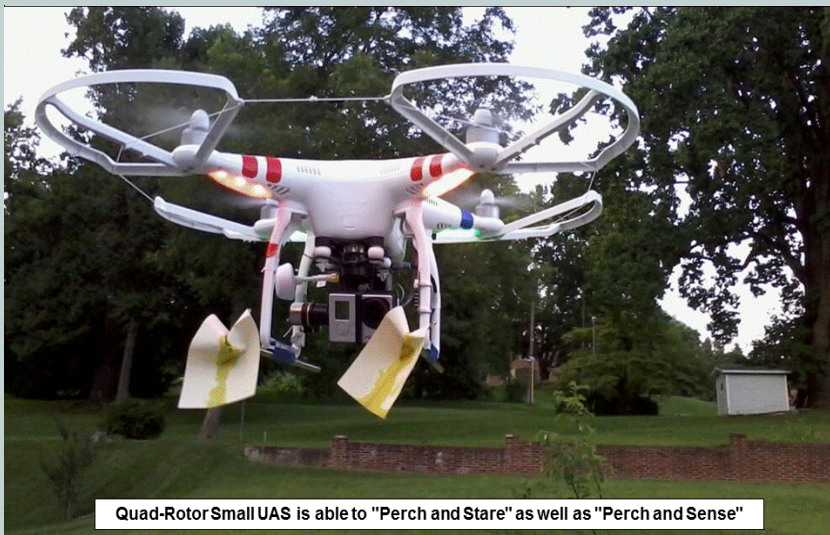
Figure 2. (Below) Rethinking M-8 Paper on a stick. On-board GPS and camera with optional LED headlights can image, transmit and record first person video streaming of real-time M-8 paper color change with stimulant used here. Funding via IR&D. (Courtesy of Science and Engineering Services/ Released)
