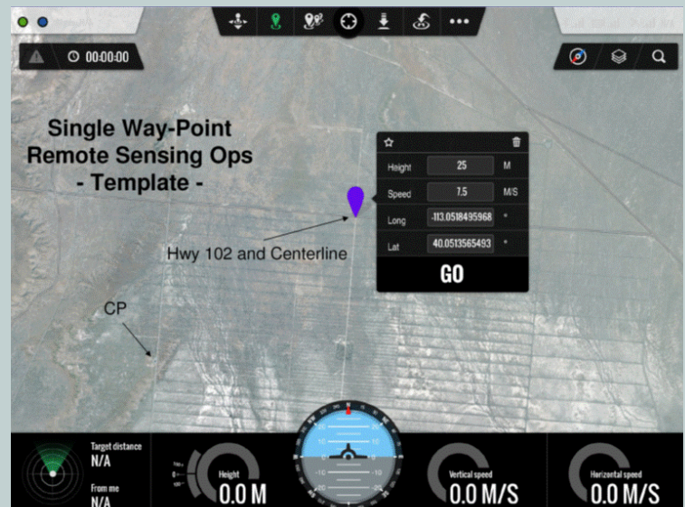
Figure 8a. Precision vectoring of quad-rotor drone from command post to way-point(s) for remote sensing and reconnaissance. (Courtesy of Dugway Proving Ground, Utah/ Released)
