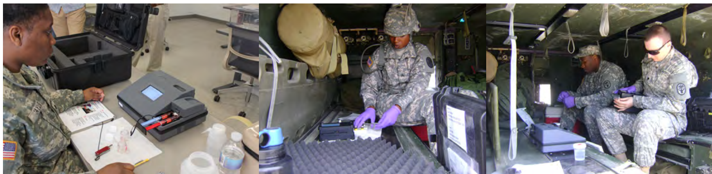
Figure 2. Soldiers performing water testing with the ESB device. Soldiers used the ESB during the customer assessment in a field laboratory setting as well as in the back of a High Mobility Multipurpose Wheeled Vehicle after transport on an off-road course.
