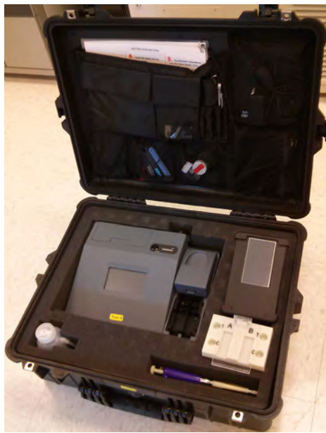
Figure 1. ECIS (instrument on the left) and ACE™ sensors (right) with reusable supplies packaged in the ESB carrying case.
