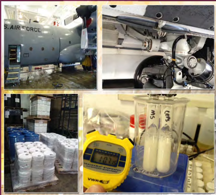
Figure 1: C-130 wash (upper left), C-17 landing gear wash (upper right), SSDX-12 manufacturing (lower left), stimulant agents remain emulsified after one hour (lower right). (Released)
