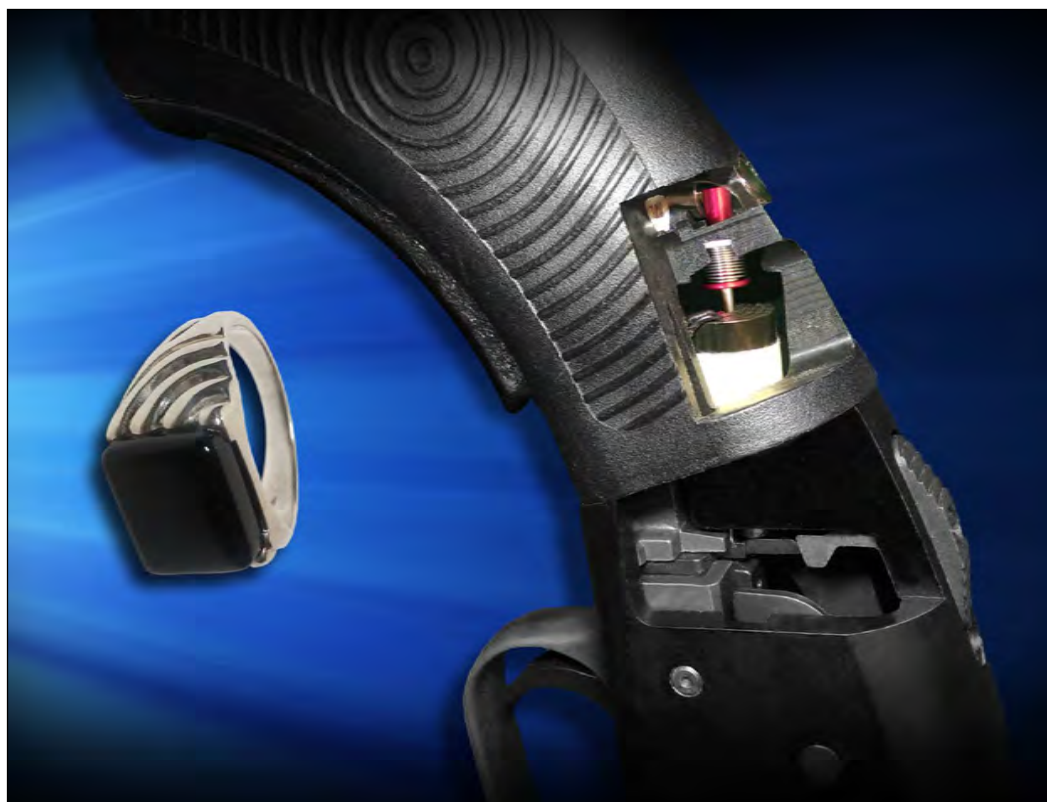
Image 3. RFID chipped ring and iGun internal disabling solenoid pictured. (Image courtesy of Jonathan Mossberg/Released)
