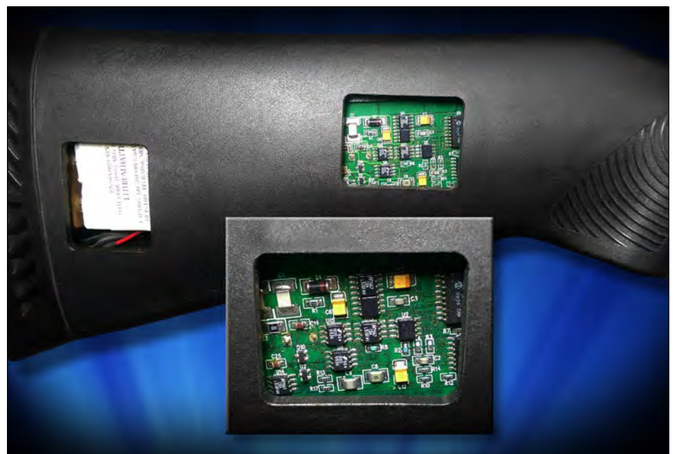
Image 2. View of the internal components of the iGun, including the battery and circuit board, enlarged view (Image courtesy of Jonathan Mossberg/Released)
