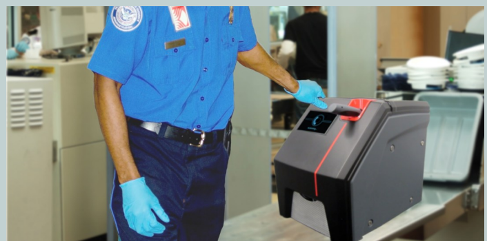
(Above and Below) Scantex proof-of-concept demonstrator in use by airport security for explosives testing. (Courtesy of Grey Innovation/Released)
