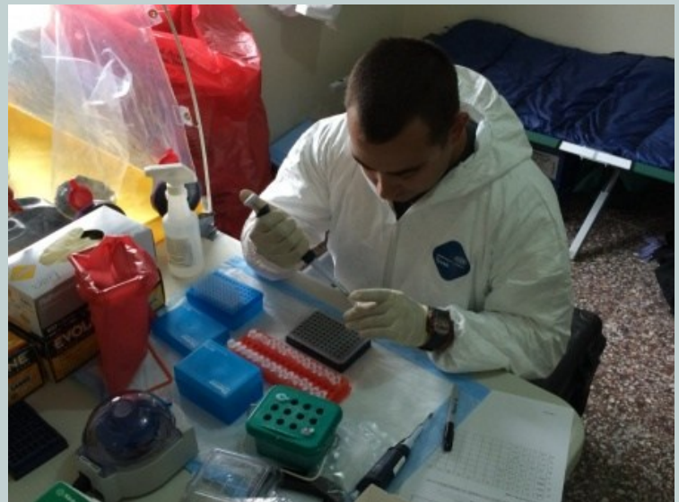
U.S. Navy Lt. Jose Garcia pipettes each patient sample into testing plate for analysis in order to identify the Ebola virus. Garcia works at a Naval Medical Research Center mobile laboratory at Bushrod Island, Liberia. The NMRC sent two mobile testing labs to Liberia to support Operation United Assistance. Each two-person lab is capable of testing up to 80 samples per day. (U.S. Army Africa photo by Chief Petty Officer Jerrold Diederich/Released)
