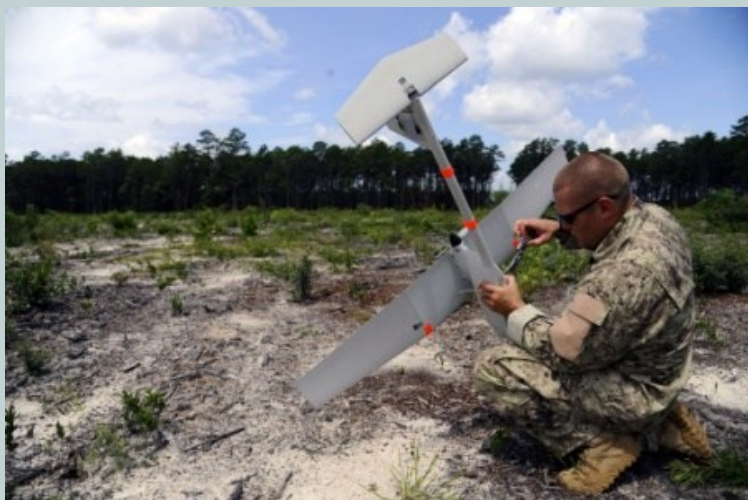
U.S. Air Force Tech. Sgt. Matthew Green fastens the GPS mechanism inside a RQ-11B Raven B unmanned aerial vehicle at the Eglin range, Fla., Aug. 9. The UAV comes equipped with a GPS in order to track the aircraft when maintaining a visual may not be possible. (U.S. Air Force Photo by Airman Gustavo Castillo/Released)
