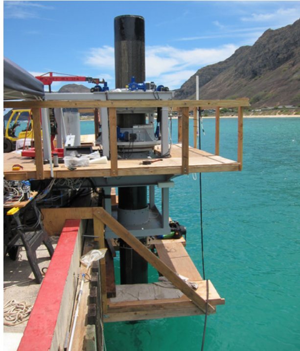
Figure 5-5. Device developed to produce deep-water pipes (Source: Makai Ocean Engineering) [80].
