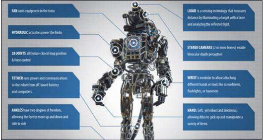
Figure 4. Overview of functions of the Atlas disaster response robot [15].
