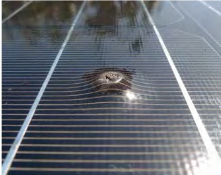
Figure 6: Ultra-light PV module after a .308 caliber ballistics test at 75 yards [22]. - (Source: Author)
