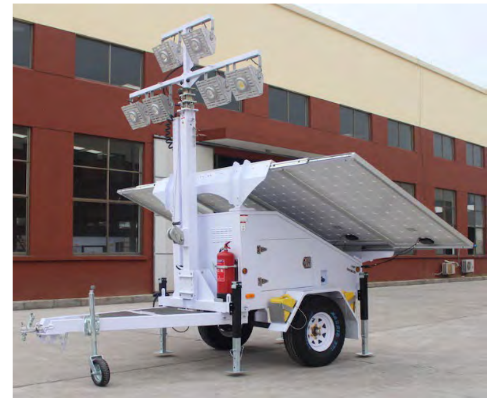
Figure 9: Battlefield Military Solar Lights Tower [14]. - (Source: Author)
