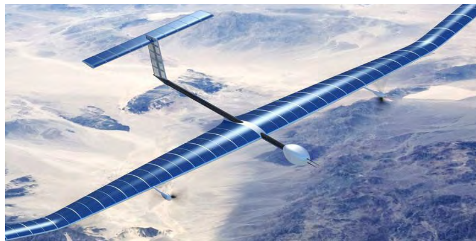
Figure 7: Zephyr High Altitude Pseudo-Satellite (HAPS) which completed a maiden flight lasting approximately 26 days without landing [10]. - (Source: Author)
