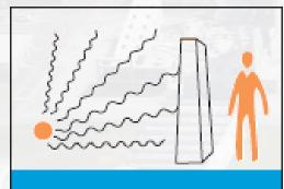
Behind shielding from source: less radiation received.
