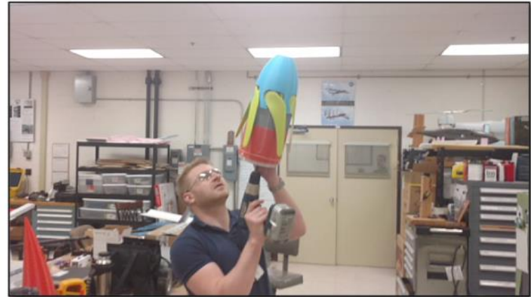
Rapid Prototype 3-d Printed Model of the Initial High Lift Folding Propeller
