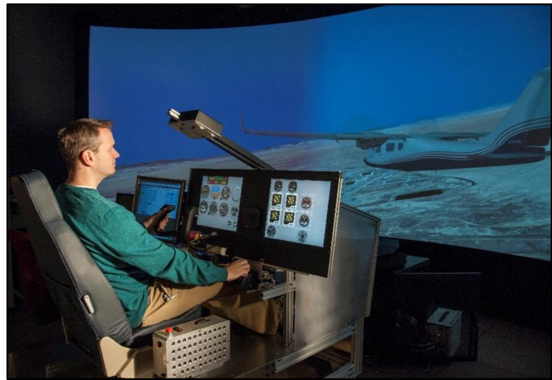
Piloted Simulator at AFRC Includes Flight Like Instrument Panels, Switches, MFD
