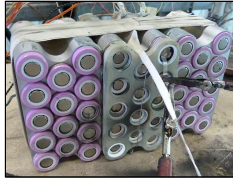
NASA JSC Test Unit With Interstitial Barrier and Heat Spreader (Design Template)
