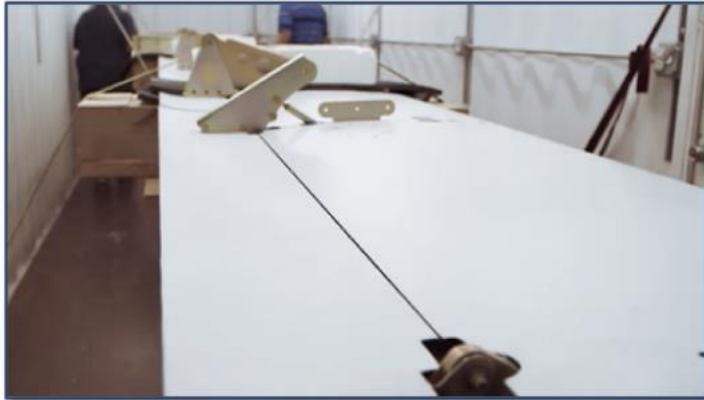
Wing Delivery and Prep for GVT and Loads Tests
