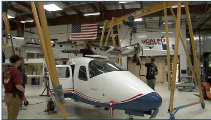
Mod II Wing installation
