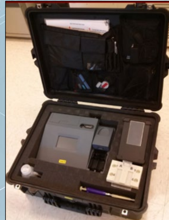
Figure 1. ECIS (instrument on the left) and ACE™ (instrument on the right) sensors with reusable supplies packaged in the ESB carrying case.
