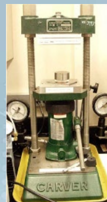
Very short path-length liquid cells to enable full dynamic range of liquid measurement made by squeezing commercial liquid cells in a press
