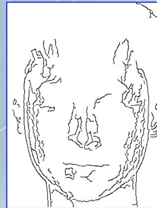
Key edges are correlated between thermal and visible facial signatures; polarization state information complements intensity-only thermal information
