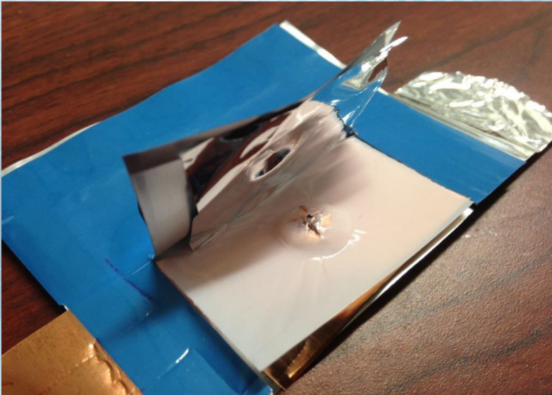
Deformation and puncture in separator
