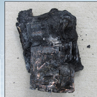
BB-2590 rechargeable battery, new (top) and after thermal runaway (bottom)
