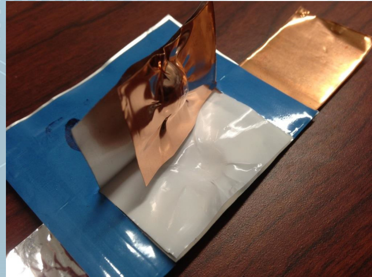
No puncture in separator
